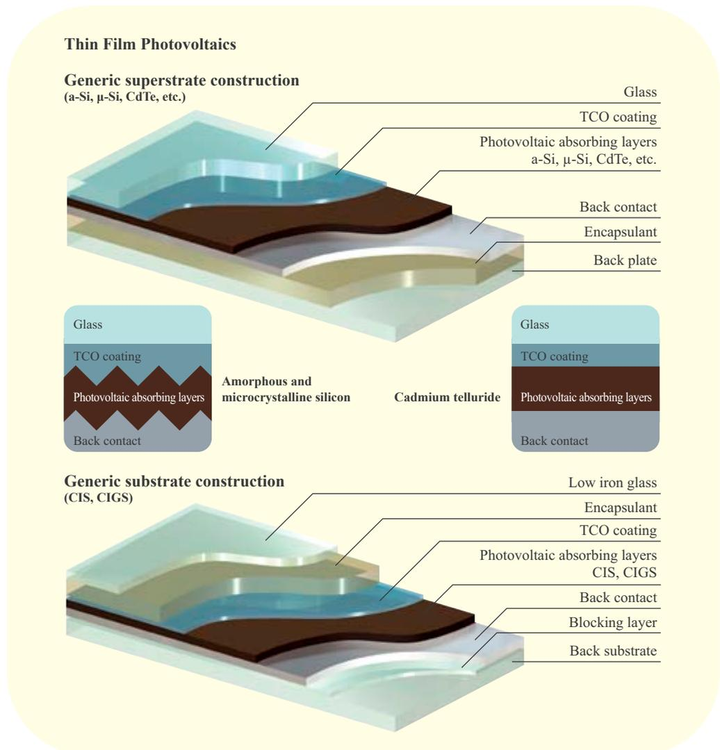
NSG **TEC™** Sodium Block is used for CIS/CIGS applications. It includes a sodium barrier layer, which offers manufacturers improved product stability and increased process throughput.
