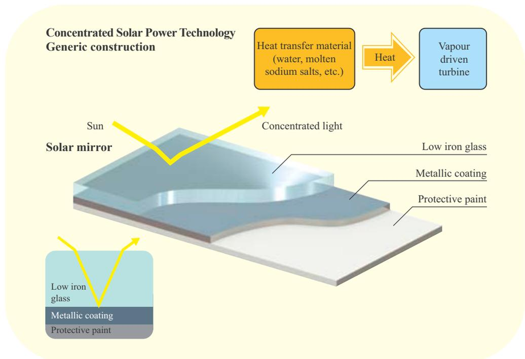
Since the sunlight has to travel through the glass twice before reaching the heat transfer material, very high light transmittance, low absorptance glass such as Pilkington **Optiwhite™** S or Pilkington **Microwhite™** is required for this application.
