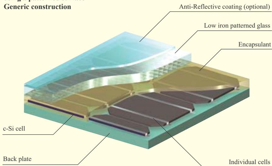
The glass type normally used for this technology is low iron rolled glass such as Pilkington **Sunplus™**, often in toughened form, combined with an Anti-Reflective (AR) coating, to ensure that the maximum solar radiation reaches the PV cells. It is also possible to use low iron float glass such as Pilkington **Optiwhite™**.
